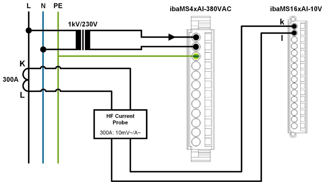
Example of 1-phase measuring with a Rogowski coil or a current clamp
