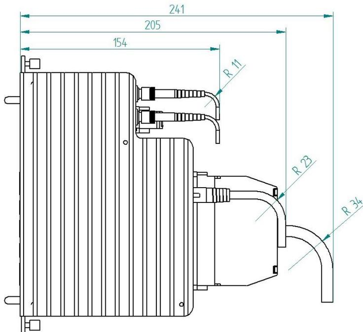
Dimensions of ibaPQU-S with cables (dimensions in mm)
