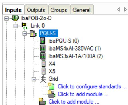
7. The current and voltage inputs required for the measurement are configured in the input modules (see chapter 8 “Measurement principles and measured quantities”).
