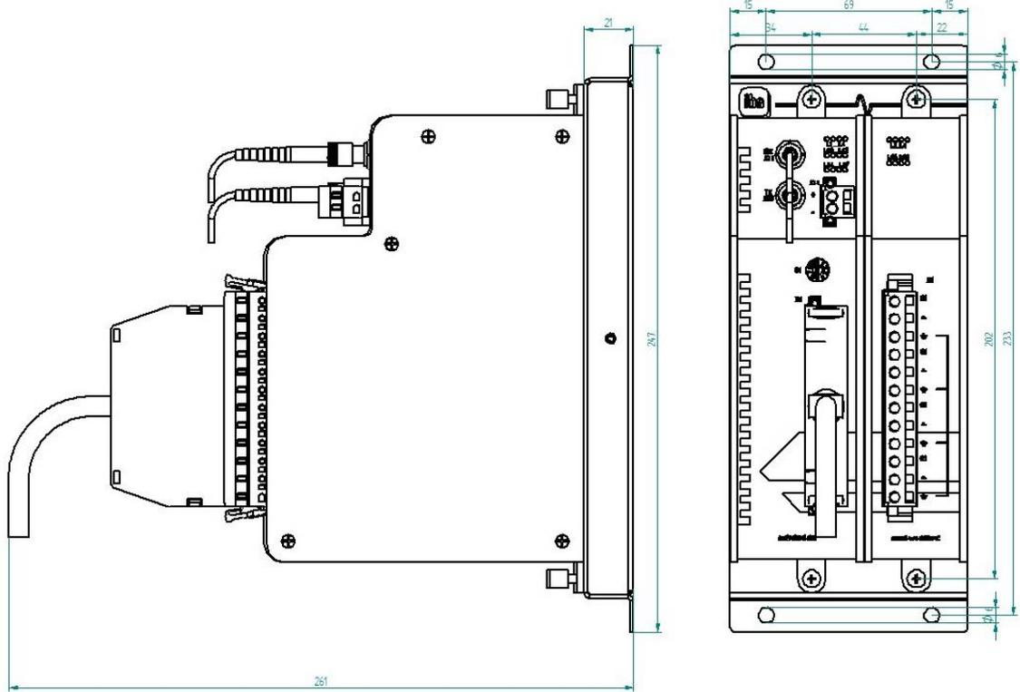
Dimensions of ibaPADU-S-B1S with modules (dimensions in mm)
